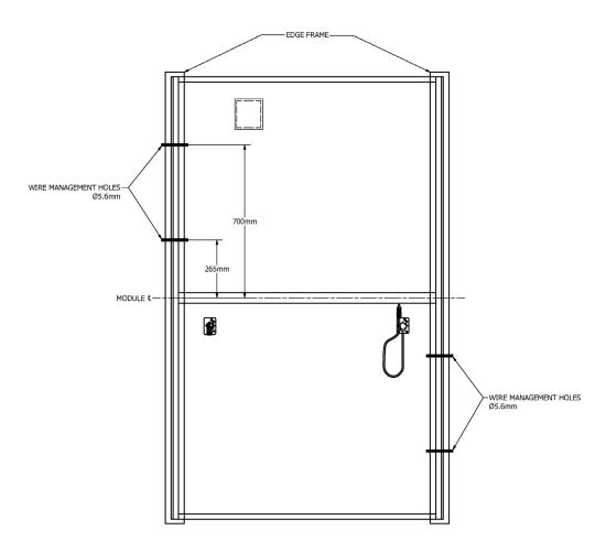
Figure 12: Frame Wire Management Hole Locations
