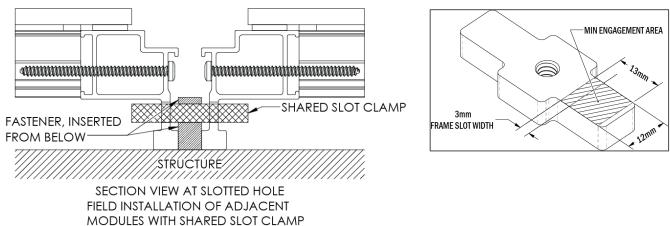
Figure 9: Shared SpeedSlot Clamp Detail
