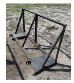
Figure 1:Example of a jig limiting forks to 1.30 m (51 in)
