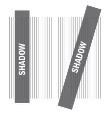
Figure 10: Example of at-risk shading patterns
