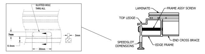
Figure 7: SpeedSlot Hole Dimensions
