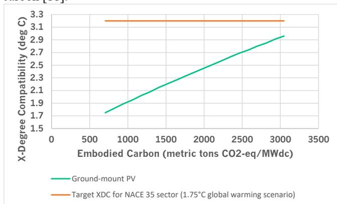
Fig. 3. Sensitivity analysis of X-Degree Compatibility with embodied carbon for 100 MWdc ground-mount PV systems in North Carolina. Lower and upper bound values for embodied carbon are from [10] and [17], respectively.
