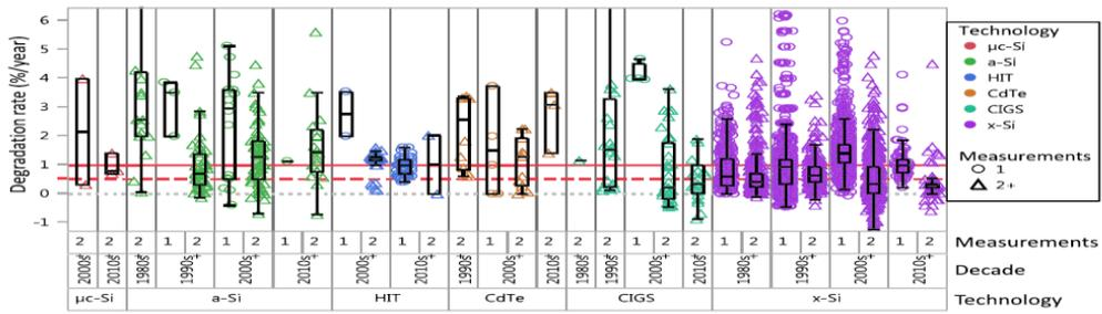
**Figure 29. Aggregation of degradation results from outdoor measurements of various PV technologies (Jordan et al., 2016).**
