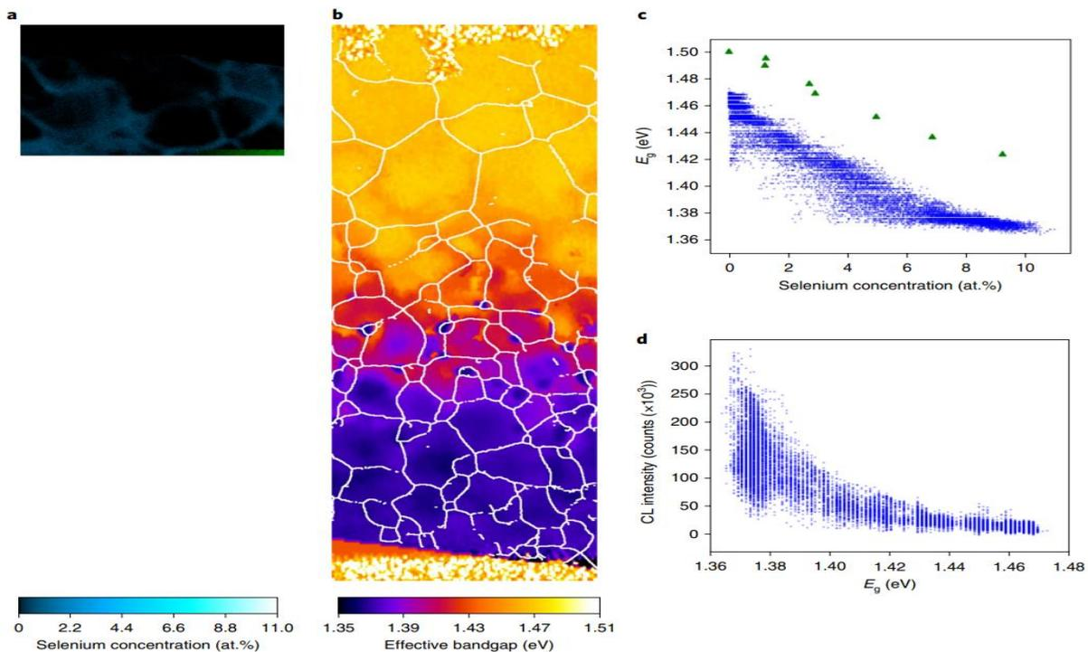
*Figure 45. A) SIMS map of the selenium concentration in a CdTe film. The selenium concentration was varied here to values between 0 and 11%. B) Shows the peak emission energy of the same film measured by cathodoluminescence (CL). This energy corresponds to the band gap of the absorber material. C) Shows the correlation between selenium concentration and band gap for all points extracted from the previous two figures. D) Shows the band gap as a function of CL (Fiducia et al., 2019).*
