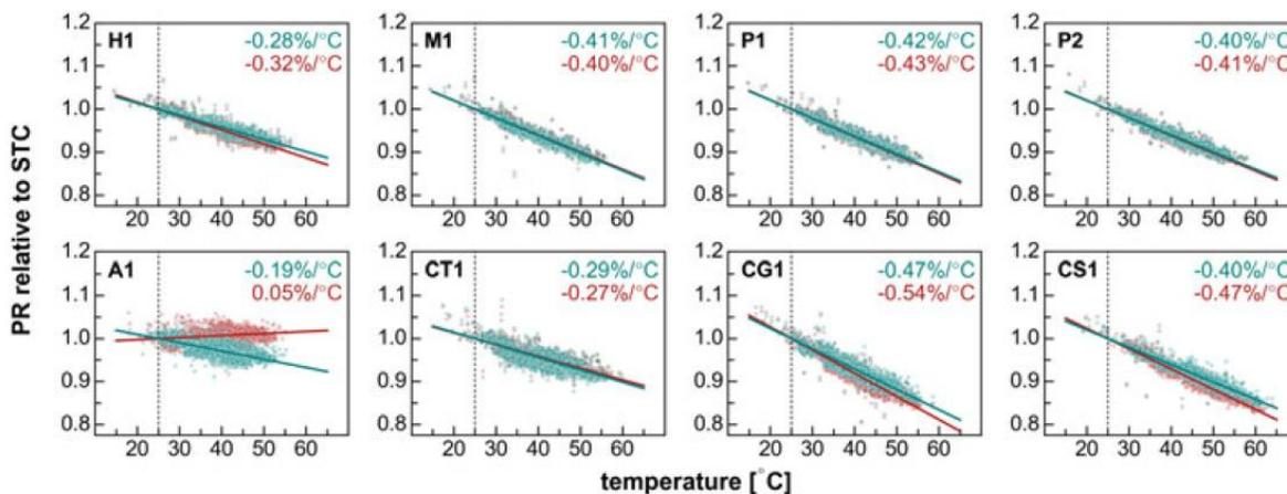
Figure 32. Examples for measured comparison of temperature effects for different module technologies for the US (A), Spain (B) and the Netherlands (C). Note that in the last figure Cadmium Telluride is abbreviated CT (Cañete et al., 2014; Strevel et al., 2012; Louwen et al., 2017).
