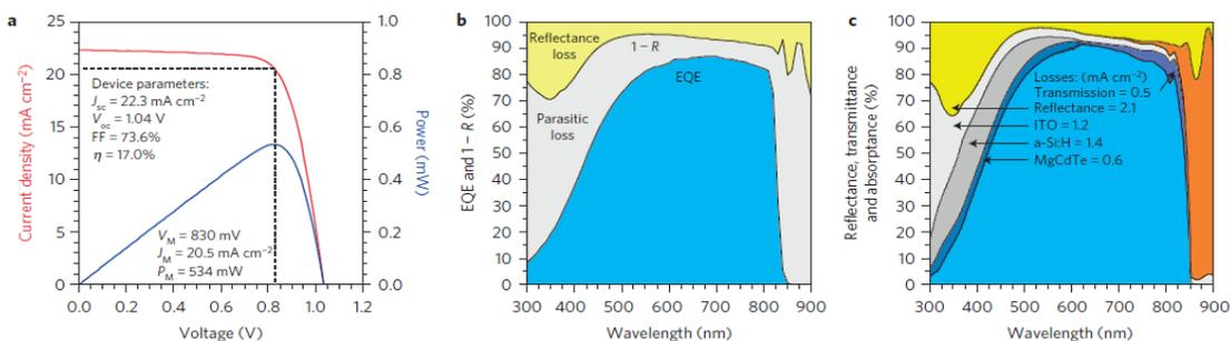
**Figure 49. A) Measured J-V curve and associated device parameters for the solar cell with structure shown. B) Measured EQE and 1-reflectance with a calculated photo-current of 22.3 mA/cm<sup>2</sup>. C) Simulated absorption spectrum for the best CdTe solar cell with a calculated photo-current of 23 mA/cm<sup>2</sup>. The improved device has a 10nm Mg<sub>0.3</sub>Cd<sub>0.7</sub>Te barrier layer (Zhao, 2016).**
