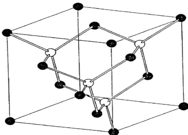
*Figure 55. Molecular structure of Cadmium Telluride with strong chemical bonding (>5 eV) (Bonnet & Meyers, 1998).*
