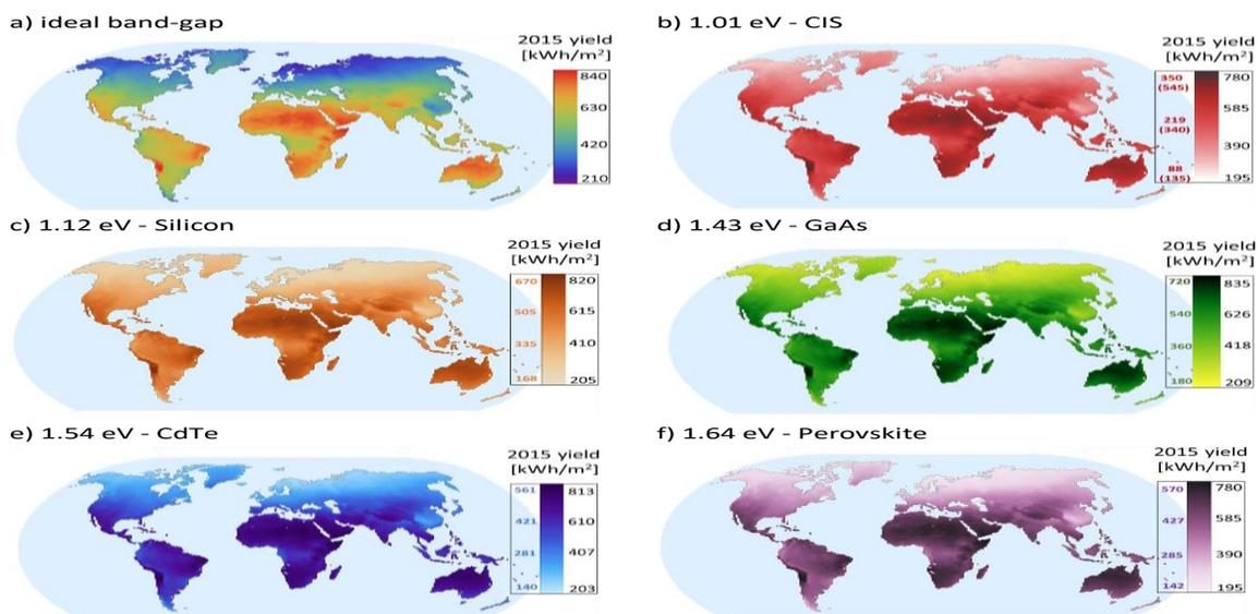
**Figure 24. (A) gives the energy yield in kWh/m<sup>2</sup> for 2015 with a material having the ideal band gap in each location. (B)-(F) show the energy yields for the five considered materials. These five graphs are shown with two axes corresponding to the radiative limit (right) and a projection to record solar cell efficiencies (left, color) (Peters & Buonassisi, 2018).**
