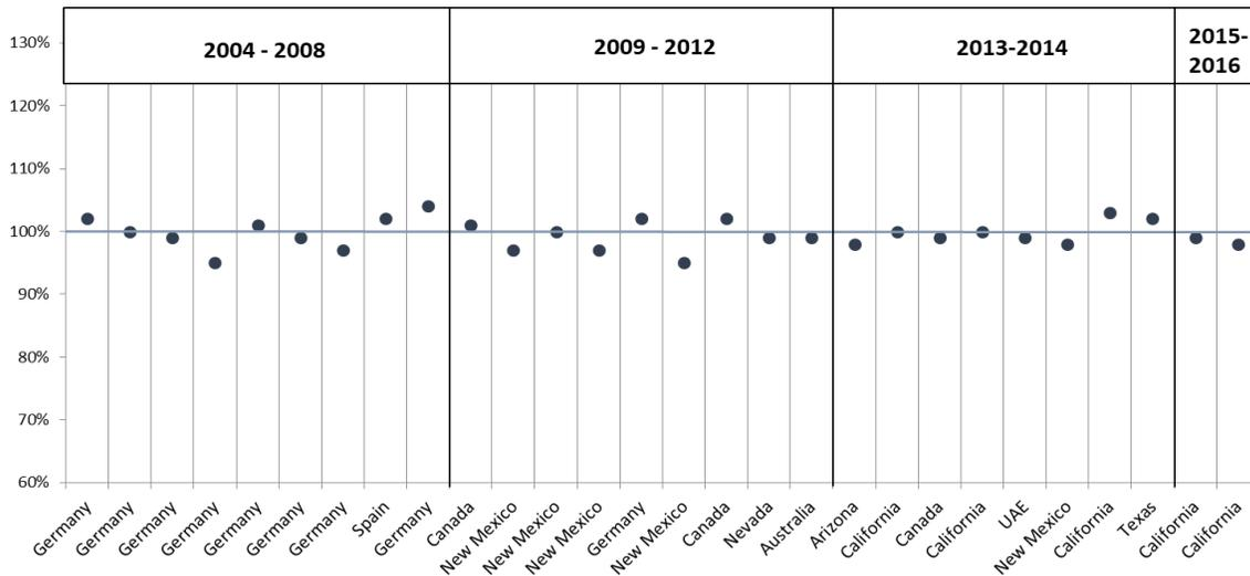
**Figure 44. Top - Voltage loss after extended light soak exposure at the maximum power point. (Strevel et al., 2013). As with S3 Black Plus, ZnTe is also utilized in Series 4 | 6 modules. Bottom - Historical predictability of CdTe PV module architecture (First Solar, 2020a).**
