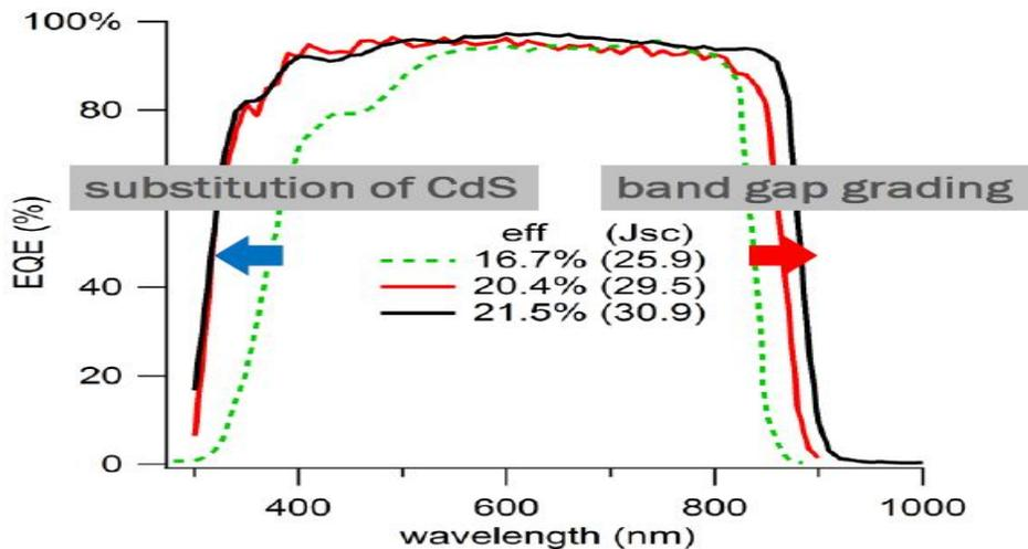
**Figure 46B.** External quantum efficiencies of different device generations. The substitution of CdS has improved the blue response of the cell, band gap grading has allowed extending the red response, together resulting in outstanding currents (close to 31 mA/cm<sup>2</sup>) and efficiencies (21.5% in this case) (Weiss, 2018).
