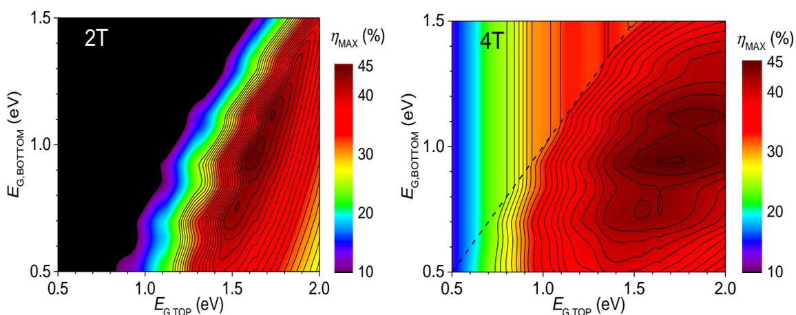
**Figure 50.** The figure on the left shows calculations for the two terminal (2T) architecture, in which the two cells are monolithically integrated, and electrically separated by a tunnel junction – making current matching necessary. The figure on the right shows the four terminal (4T) architecture, in which the two cells are contacted independently and only optically connected (Mailoa, 2016).
