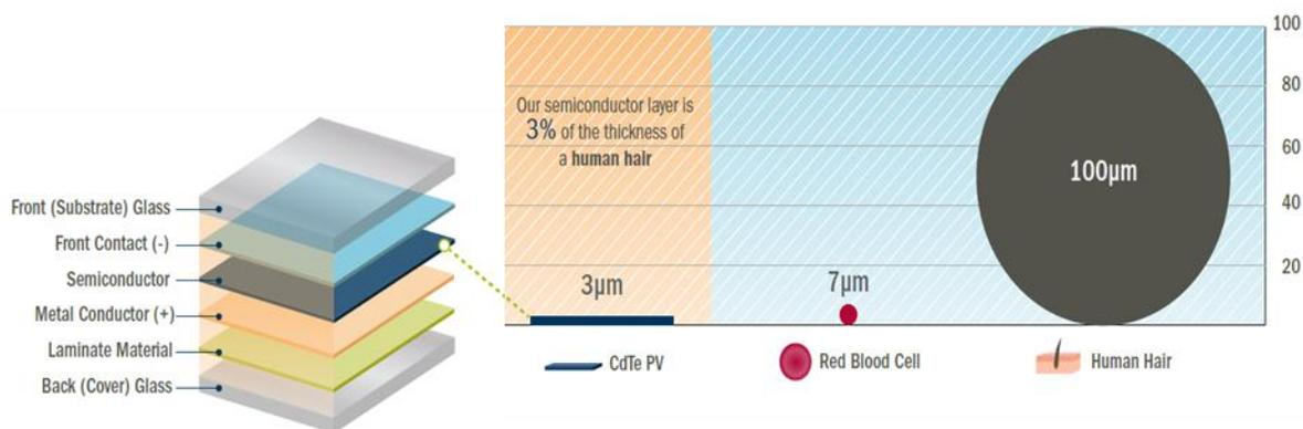
*Figure 61. In the PV module structure, the CdTe semiconductor is a 3-micrometer thin film sealed between two glass layers (First Solar, 2018).*
