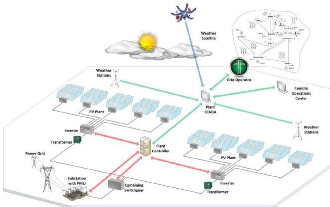
**Figure 97 Components of a typical utility-scale PV power plant. Image from NREL (Gevorgian & O'Neill, 2016).**
