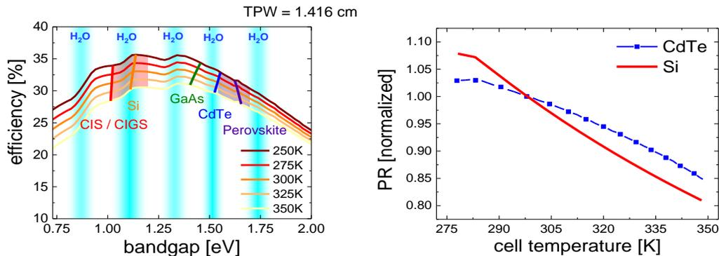
Figure 16. Left - Limiting efficiency as a function of band gap and temperature. Band gaps of various PV technologies as a function of temperature are also shown. Right - Normalized performance ratio of a CdTe PV module and PERC-type silicon solar cells. CdTe is less sensitive to changes in temperature and has a comparably higher performance ratio at high temperatures (Peters et al., 2018)
