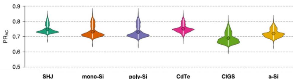
**Figure 21A. Simulated performance ratios for a variety of solar cell technologies for all areas shown in B.**
