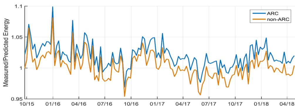
**Figure 37. Ratio of average weekly measured to predicted power generation of a group of modules with (blue) and without (orange) anti-reflective coating (ARC) (Passow, 2018).**
