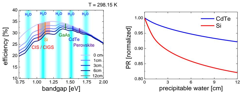
**Figure 18. Left - Limiting efficiency as a function of band gap and total precipitable water. Band gaps of various PV technologies are also shown. Right - Normalized performance ratio of a CdTe PV module and a PERC type silicon solar cells as a function of total precipitable water (Peters et al., 2018)**
