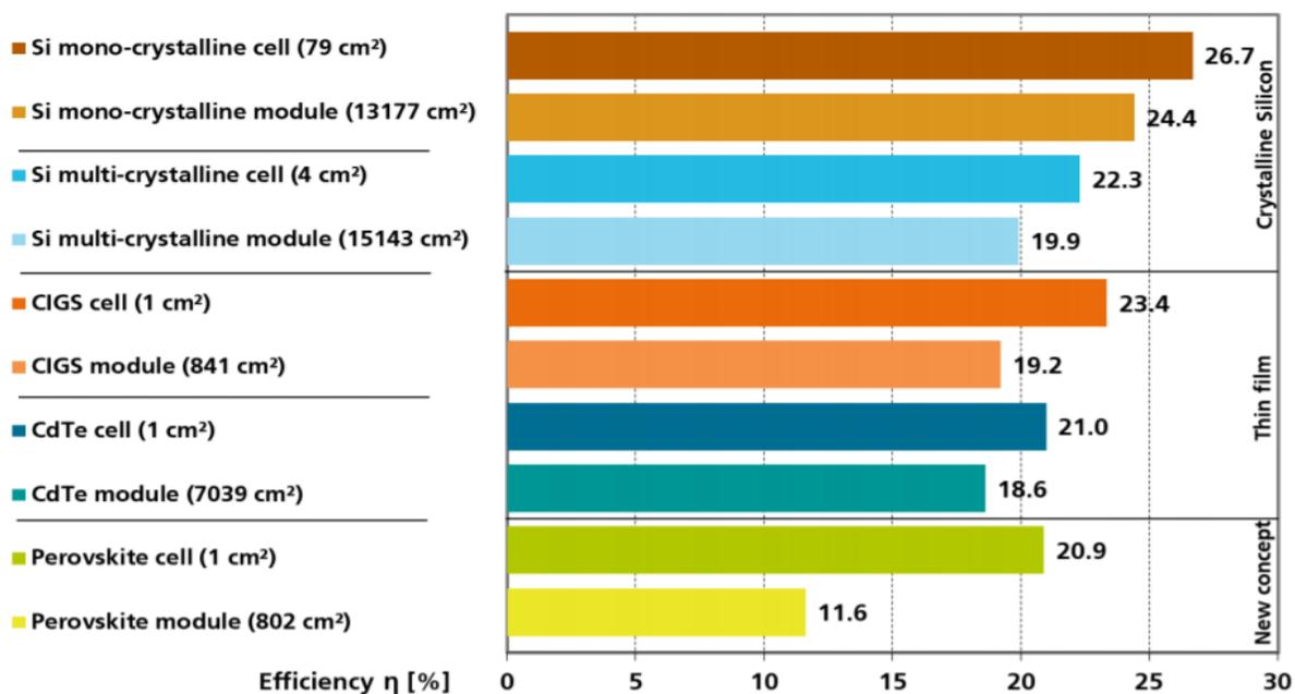
Figure 8. Comparison of state-of-the-art research cell and module efficiencies for a variety of different PV technologies (Fraunhofer, 2019).
