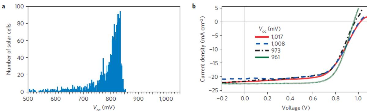
**Figure 47.** Burst et al. (2016) show how new concepts can overcome historical barriers of CdTe solar cells. A) Shows a histogram of VOC values measured at NREL for more than 2400 devices. No devices much above 850 mV appear in this chart. B) New developments have enabled CdTe to surpass the 1V barrier.
