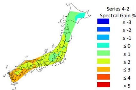
Figure 19. Irradiance rated spectral gain in energy yield for the First Solar series 4-2 module in different regions of the world (Lee et al., 2015).
