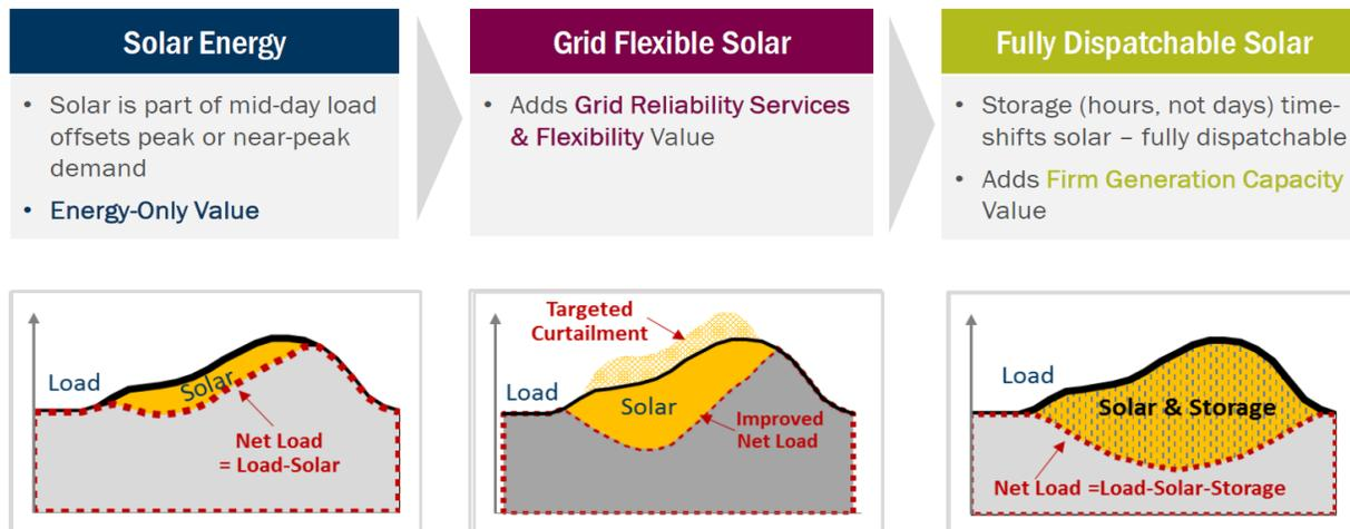
Figure 103. Progressing from simple PV deployment over grid flexible solar to fully dispatchable solar. (Morjaria, 2018).
