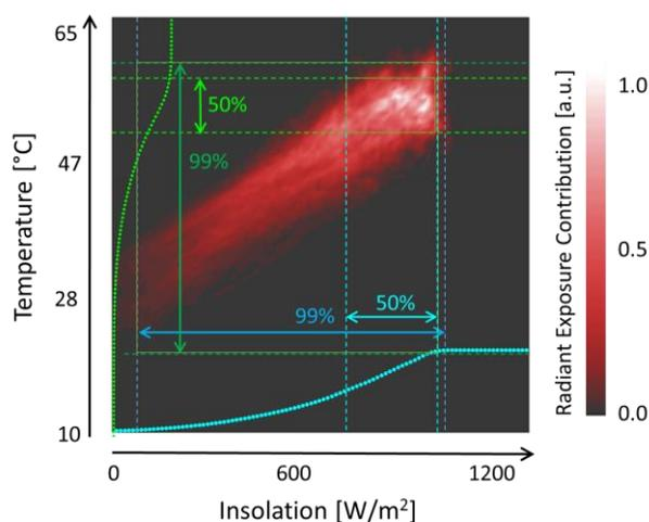
**Figure 17. Insolation and module temperature in a hot and arid sub-tropical environment. The majority of the power is generated at module temperatures between 50 °C and 60 °C (Peters et al., 2018).**
