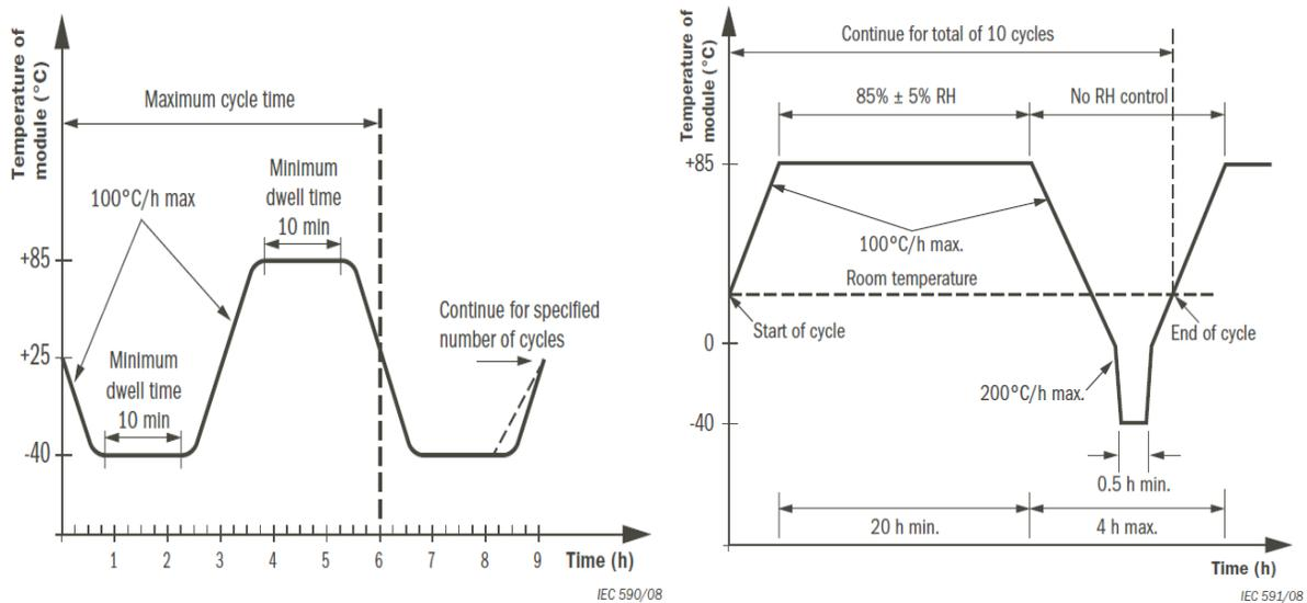
**Figure 40. Left - IEC 61646 thermal cycling profile. Right - IEC 61646 humidity freeze profile (Strevel et al., 2013).**
