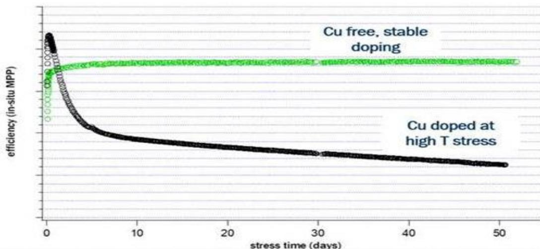
**Figure 31. Recent results about a strategy to eliminate the consolidation phase in new First Solar CdTe modules (Metzger et al., 2019).**
