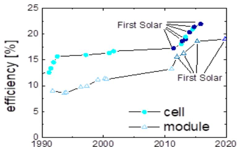
Figure 7. Development of cell (dots) and module (triangle) record CdTe PV efficiencies over the past 30 years. First Solar's contributions are marked by darker shades (National Renewable Energy Laboratory, 2019).
