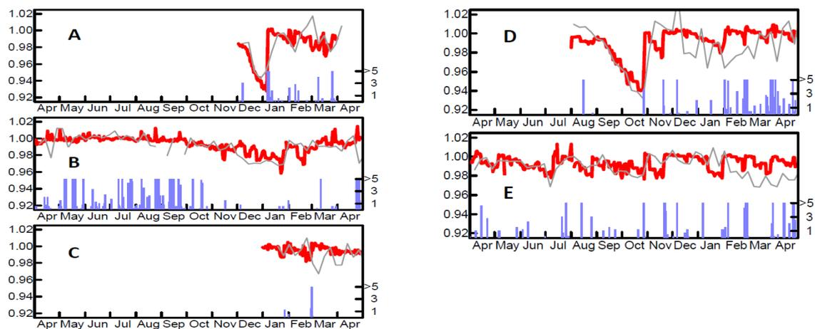
**Figure 38. Daily ratios of effective irradiance (insolation) received by soiled to non-soiled modules (soiling ratios) over time (thick line), as well as normalized power output (thin line) over one year (2013 / 2014). Blue bars indicate rainfall (Gostein et al., 2014).**
