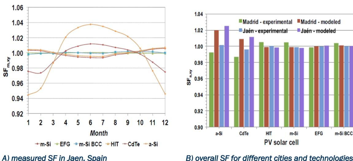
**Figure 33. A) Measured spectral factor (SF) over the course of a year in Jaen (Spain). B) Experimental and simulated results for the overall SF in Madrid and Jaen. (Alonso Abella et al., 2014)**
