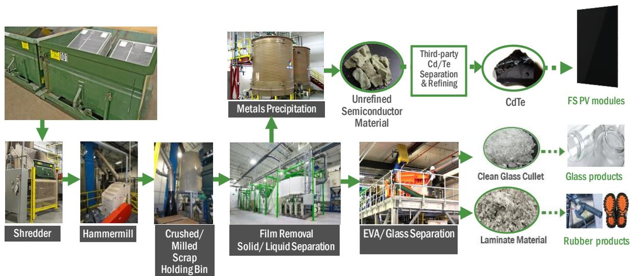
*Figure 72. First Solar’s recycling process flow (Version 3) (2019).*
