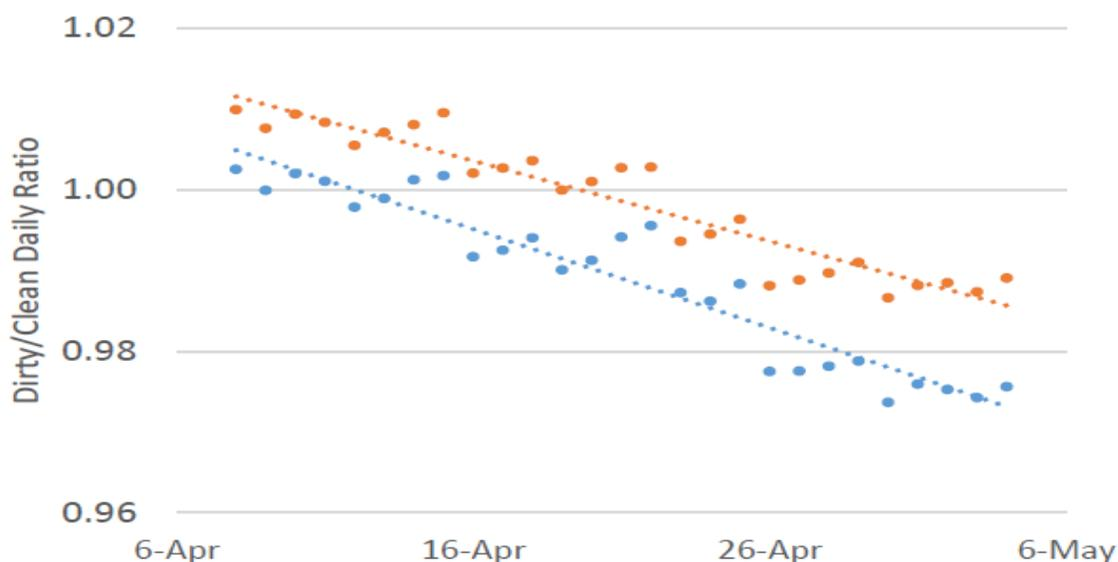
*Figure 39. Soiling trends observed throughout Spring 2015. Blue circles are daily ratios of dirty to clean insolation for First Solar non-ARC CdTe modules, orange circles are daily ratios of dirty to clean insolation for First Solar ARC CdTe modules. The soiling rate of each data set is determined by the slope of each dotted line (Grammatico & Littmann, 2016).*
