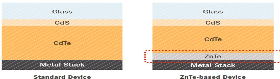
Figure 42. Solar cell architecture without (left) and with (right) ZnTe back contact. (Strevel et al., 2013).
