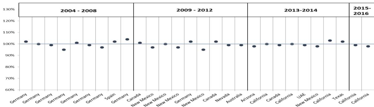
**Figure 27. Comparison between the measured and predicted lifetime performance of First Solar PV systems by commissioning date (Buehler, 2015).**
