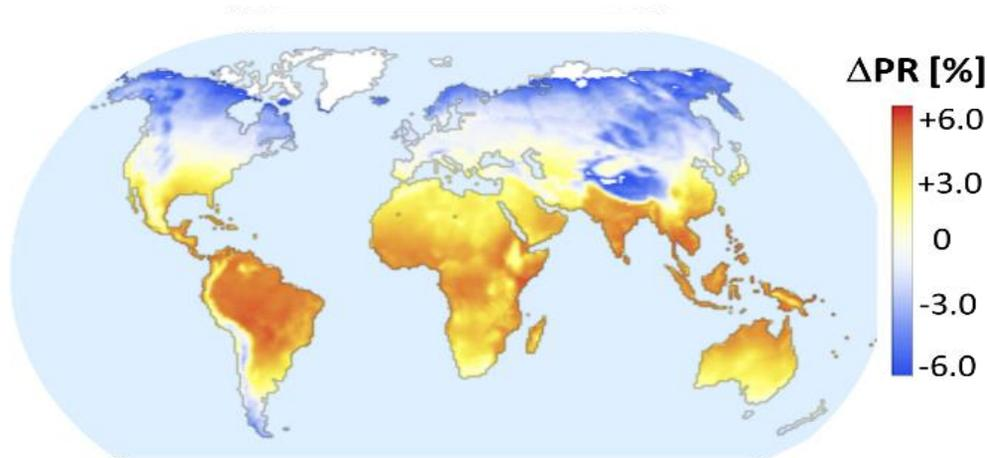
**Figure 22. Calculated annual average performance ratio difference between a silicon PERC solar cell and a CdTe PV modules. Positive values, indicated by red and yellow tones, mark a performance advantage for CdTe, blue values one for Si (Peters et al., 2018).**
