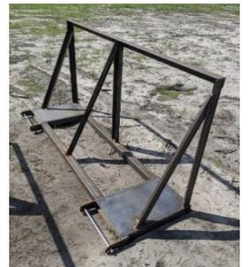
**Figure 1:** Example of a jig limiting forks to 1.30 m (51 in)
