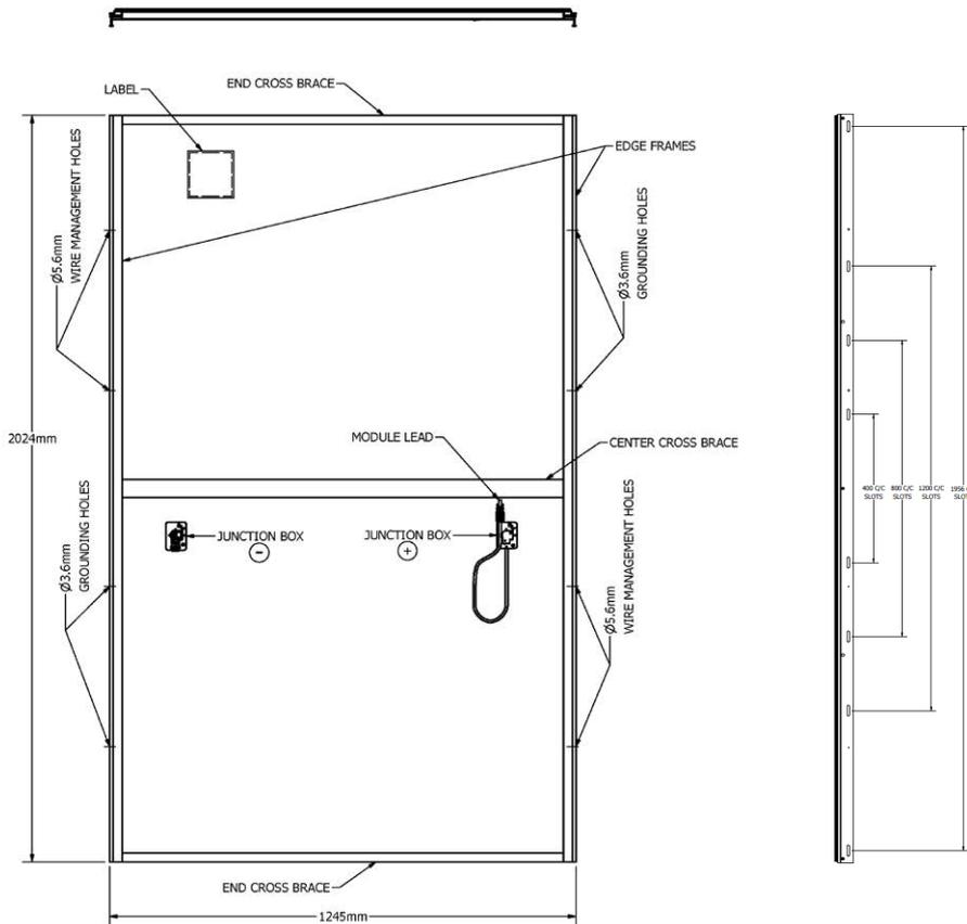
Figure 5: Series 6 Plus Module Mechanical Drawing Showing the Backside
