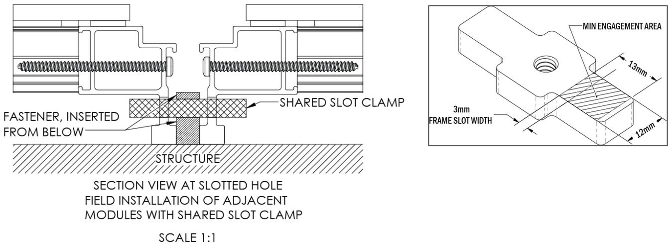
Figure 9: Shared SpeedSlot Clamp Detail
