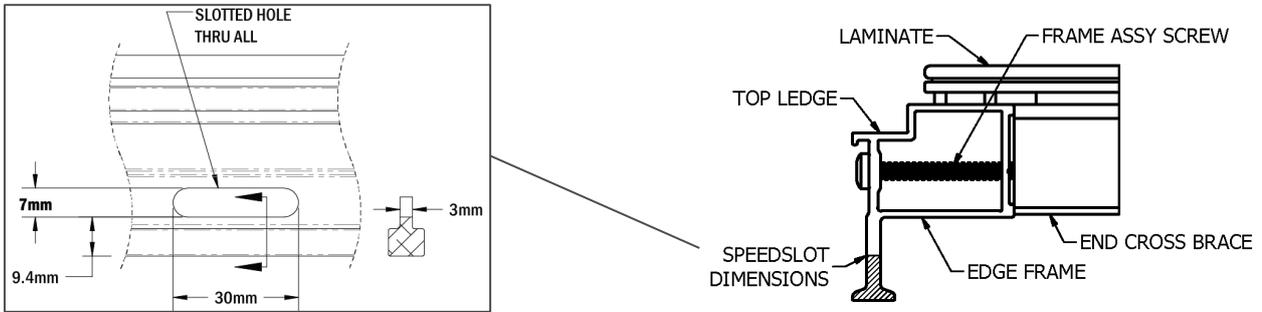
Figure 6: SpeedSlot Dimensions
