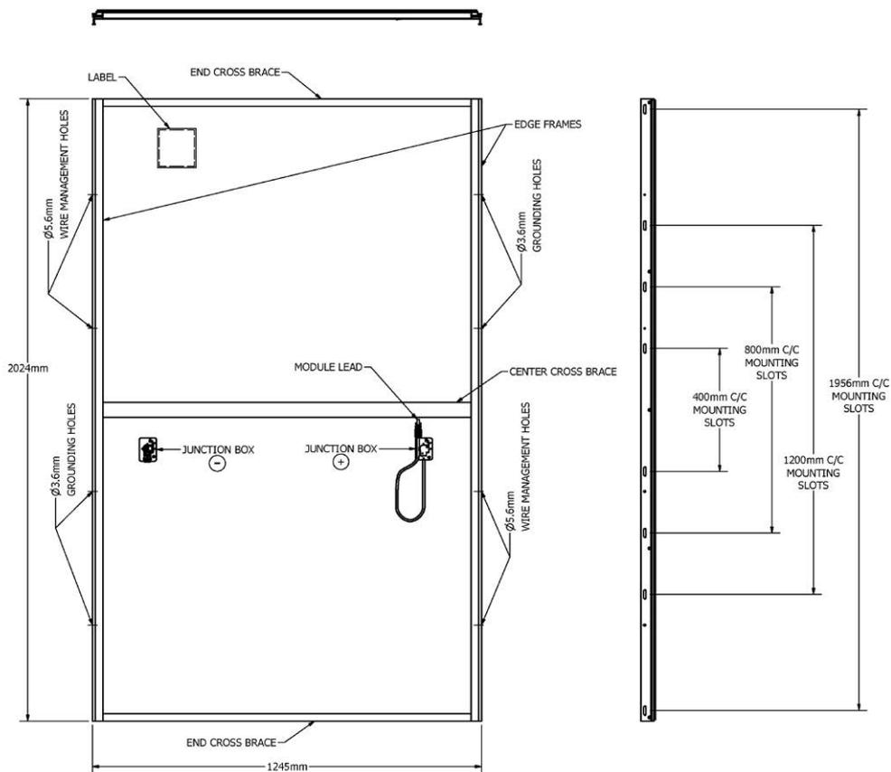
**Figure 4:** Series 6 CuRe Module Mechanical Drawing
