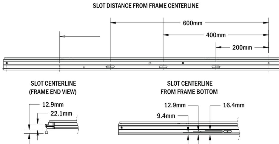
Figure 7: SpeedSlot Detail on Long Edge Frame
