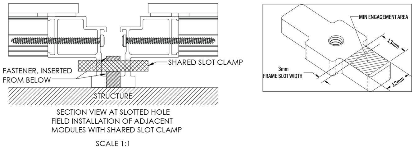
Figure 8: Shared SpeedSlot Clamp Detail
