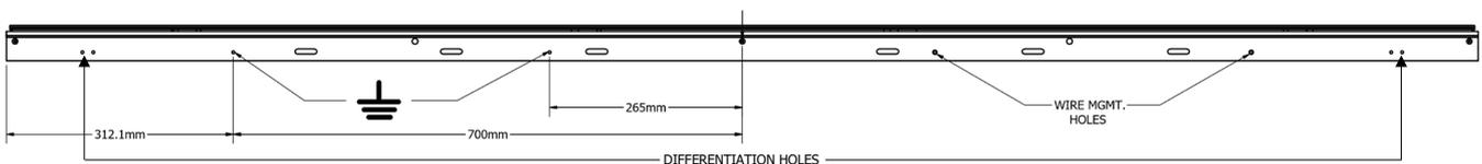
**Figure 10:** Grounding Hole & Wire Management Hole Detail from Frame Center<sup>7</sup>
