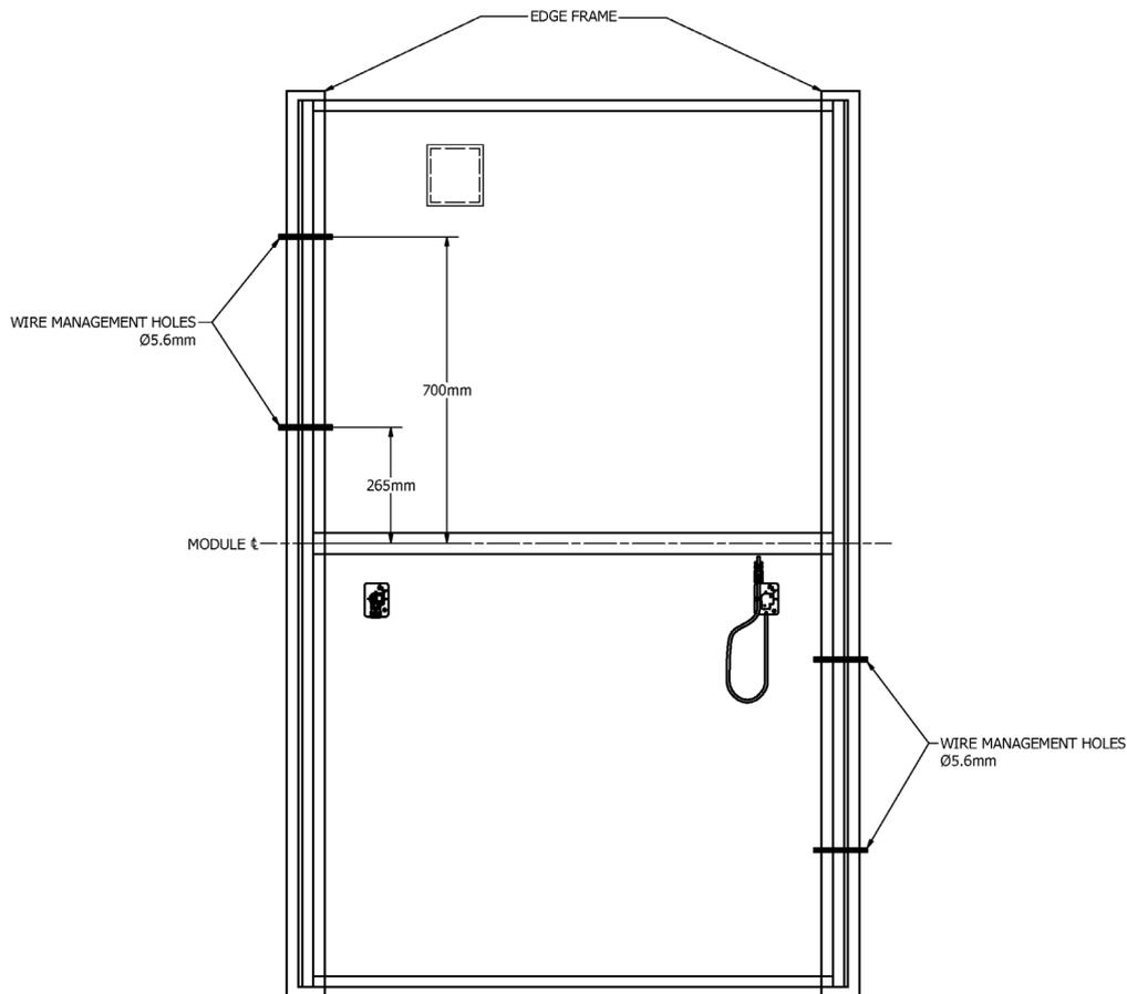
**Figure 11:** The above-ground DC cabling (typically a bundle of harnesses and PV array cables) may be supported by the wire management holes located on the Series 6 CuRe module edge frames.
