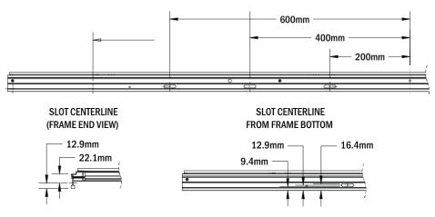
Figure 7: SpeedSlot Detail on Long Edge Frame
