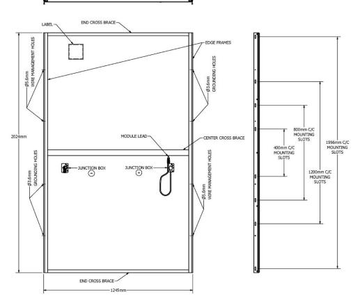
Figure 4: Series 6 CuRe Module Mechanical Drawing
