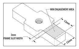
Figure 8: Shared SpeedSlot Clamp Detail
