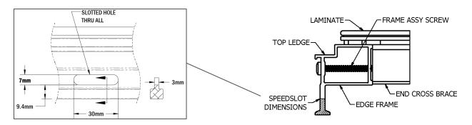
Figure 6: SpeedSlot Dimensions
