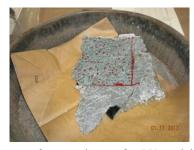
Fig. 6. Compactor foot punch-out of a PV module crushed in a Municipal Solid Waste Landfill in the State of Arizona, USA.
