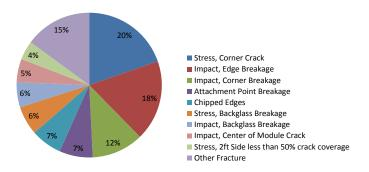
Fig. 3. PV module breakage types from warranty return data for modules put into operation (1-113 months in service).
