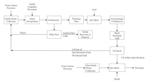
Figure 9 Wastewater treatment process flow diagram
