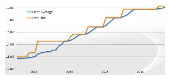
Figure 10 First Solar CdTe module efficiencies roadmap
