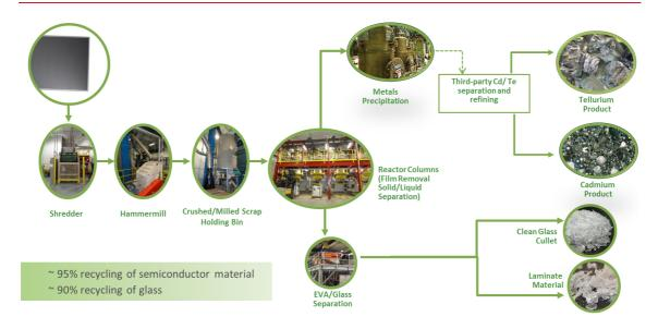
Figure 4 First Solar's module recycling technology version 2
