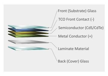
Figure 2 Schematic representation of First Solar module architecture 12
