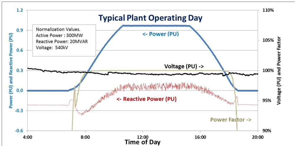
Figure 11 Normal Daily Operation of 290 MW PV Plant
