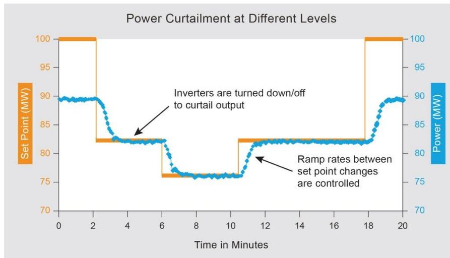
Figure 3 Power Curtailment at different levels
