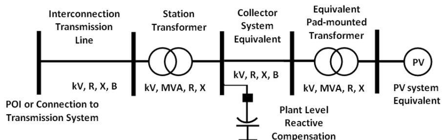
Figure 6 Single-machine equivalent load flow representation
