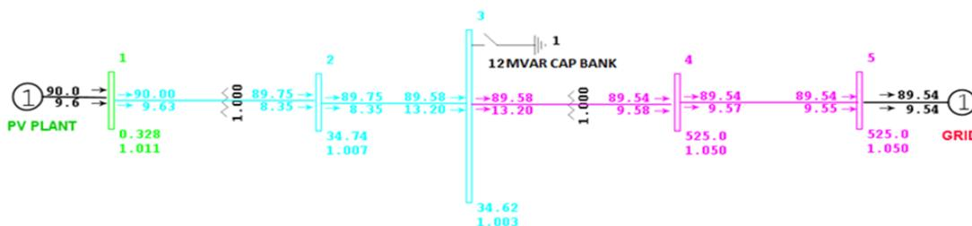
Figure 7 PSLF Equivalent Model for plant under test
