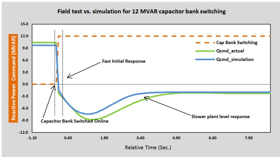
Figure 8 Qcmd response Field Test vs. Simulation
