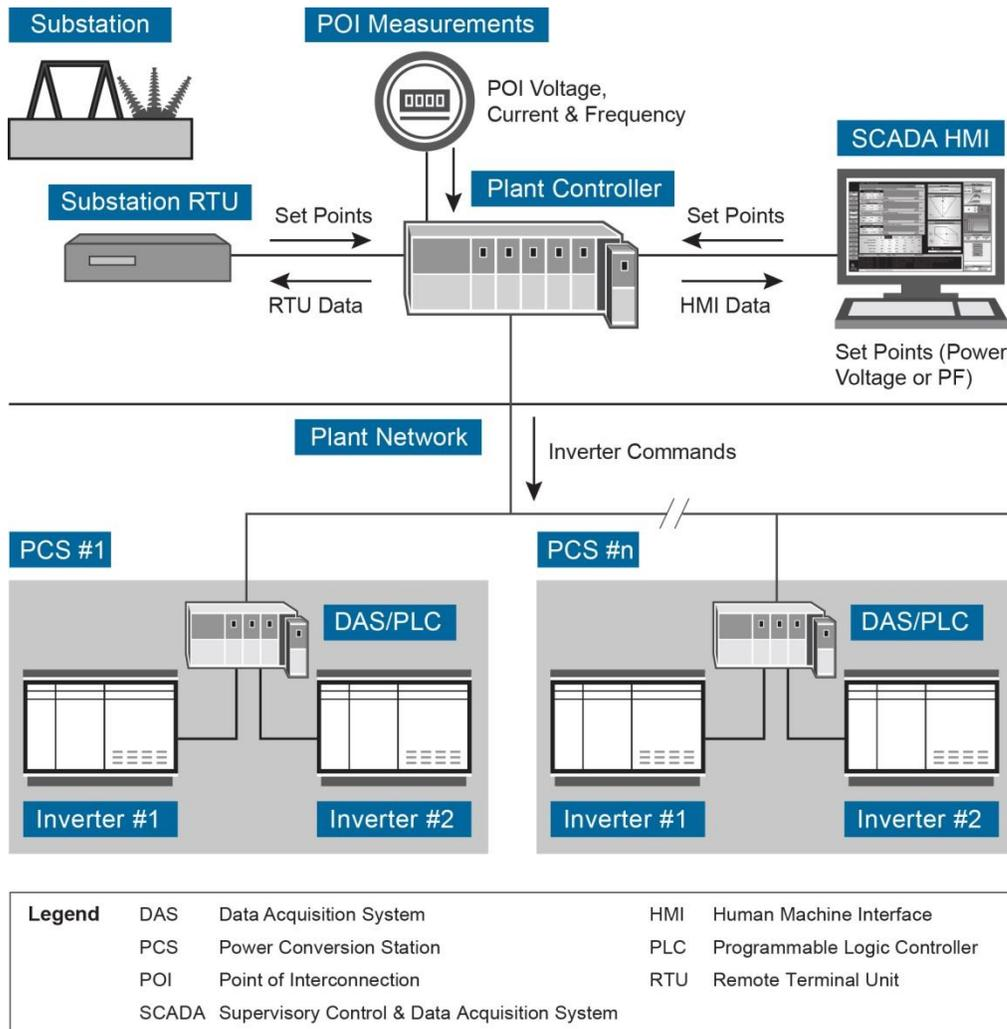
Figure 2 Plant Control System and Interfaces to Other Components
