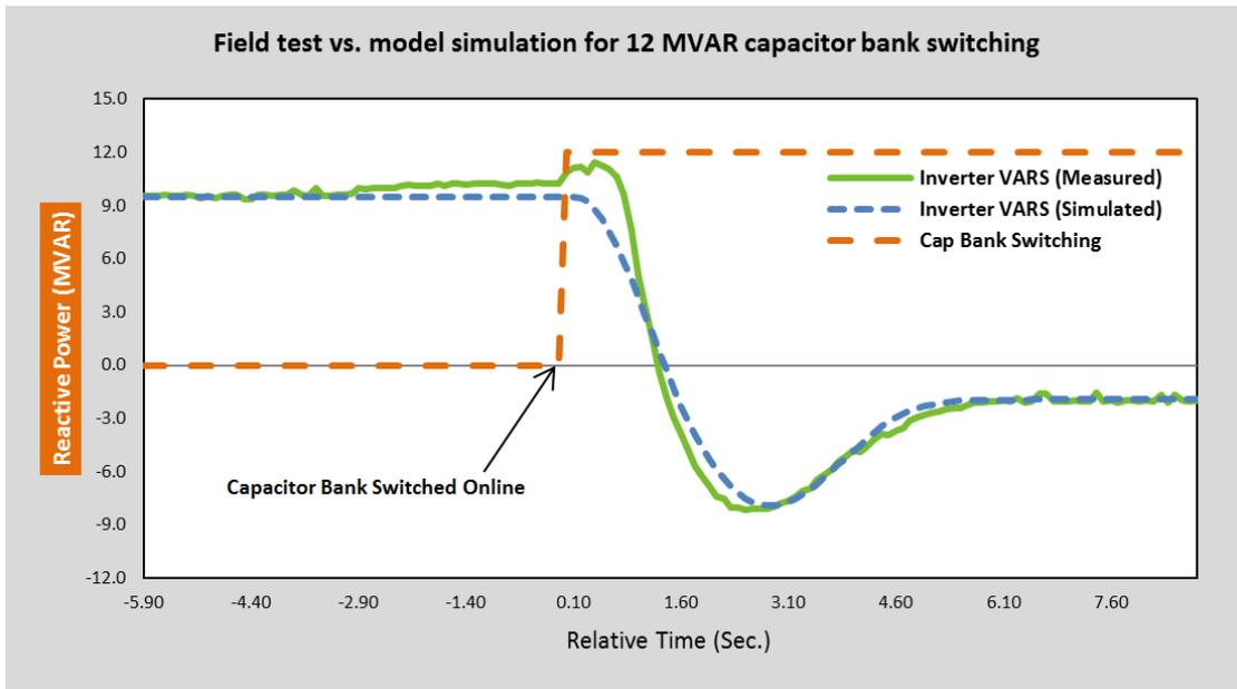
Figure 9 Inverter VARs during 12 MVAR Cap bank switching test
