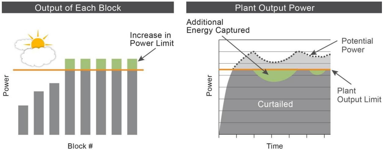
Figure 4 Impact of Cloud Passage under Curtailment
